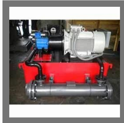
Hydraulic Power Pack
